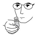
Post-analysis sterilization is performed by exerting gentle pressure on the cap and allows the safe disposal of the vial.
